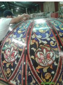
Dome frame rests on the framed in ring of the light box (by others). If you wish to hang the dome, cables may be attached to the threaded anchors to hang frame to the ceiling of light box (typically 1/8" cable).
